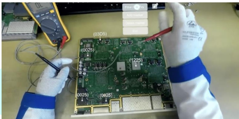
Fig: A technician repairs a circuit board using an augmented reality overlay at Ericsson's Tallinn factory.
