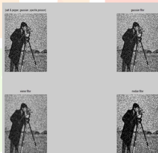
Fig 4.1: The input image (cameraman.tif) is noised with combination of all the 4 noises i.e (salt & pepper + Gaussian + Speckle + Poisson) noise. Here the noisy image acts as an input image to the filters. Noise is added externally to note the changes. The noised image is denoised using Gaussian, wiener, medianfilter
