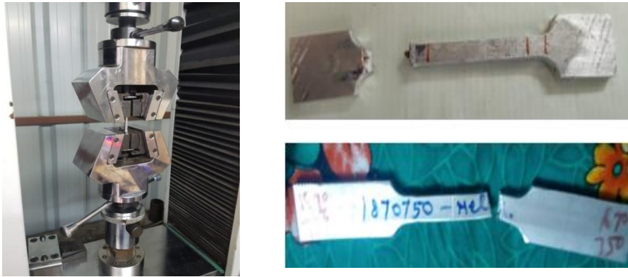
Fig .2: Testing of Metal Matrix Composite and Al- 6061 using UTM
