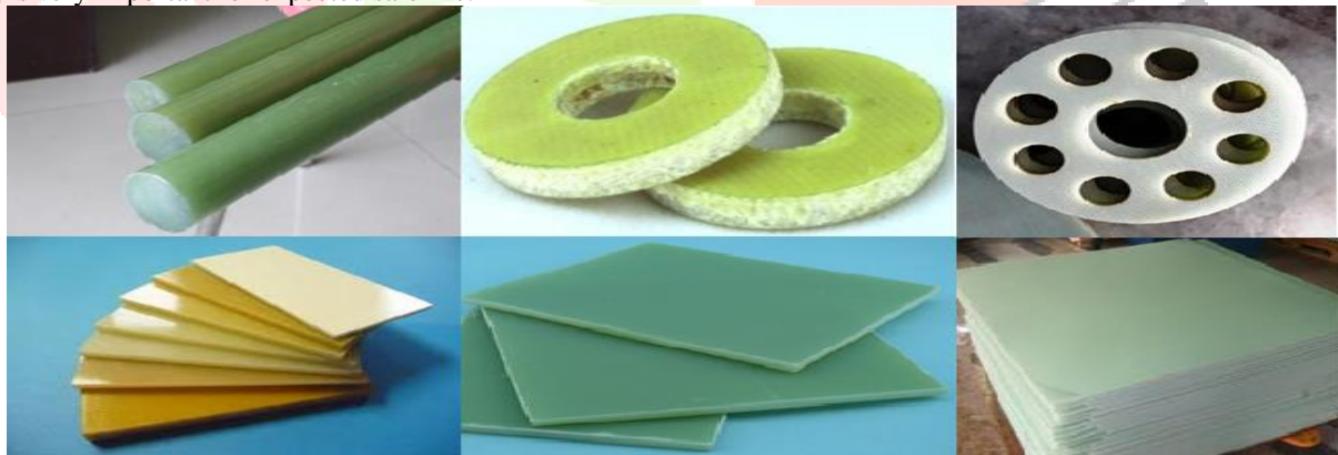
Figure-2 Different electrical insulators parts of composite materials for experiments
