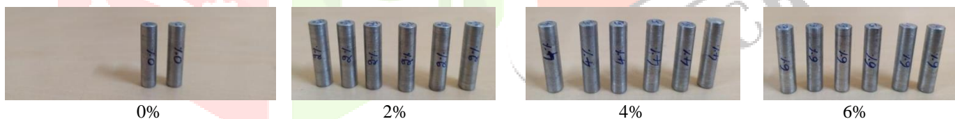
Fig 3: Wear specimen of AA 6063 MMC with TiC , 0%, 2%, 5%, 6%.
