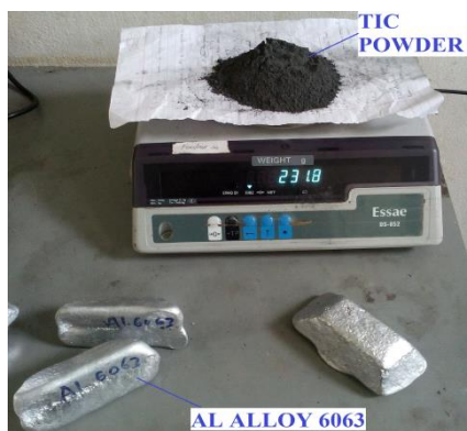
Fig 1: Aluminium alloy sample and TiC powder
