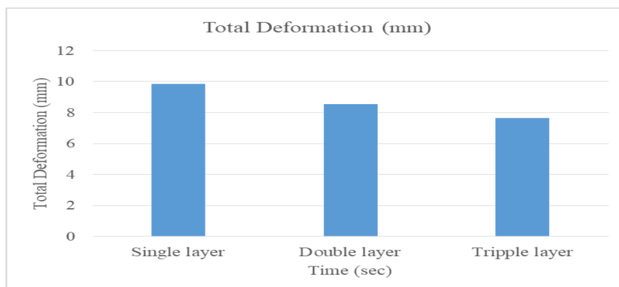
Graph 10: Total deformation in single, double and triple layer
