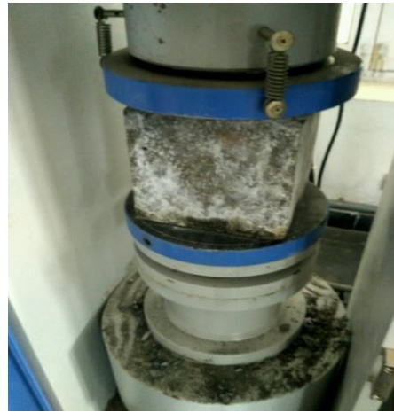
Fig 3.1: Compressive Strength Test
