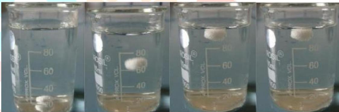
Fig 4: Floating tablets of Esomeprazole in 0.1 N HCl
