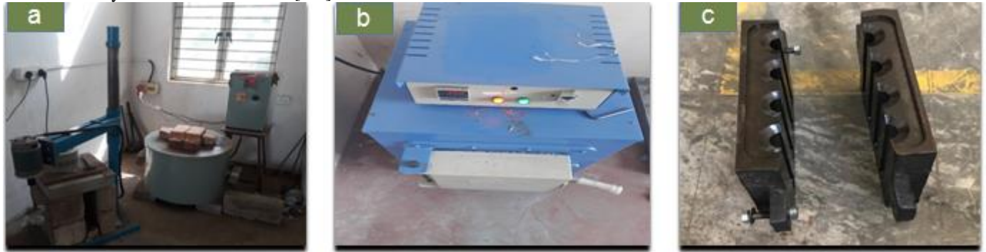
Fig 3.a & 3.b: Muffle furnace used for heating aluminum alloy Fig 3.c: Dies
