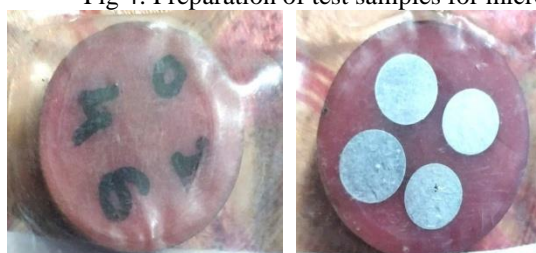
Fig 5: Etched samples for microstructural analysis of 0%, 2%, 4%, 6% TiC with AA6063
