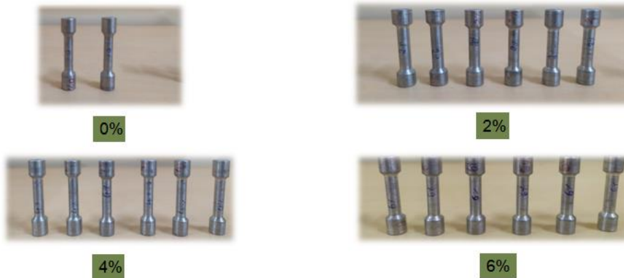
Fig 8: Prepared test samples as per ASTM-8
