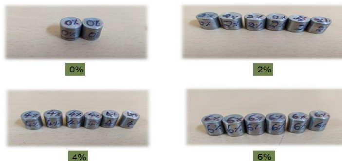
Fig 4: Preparation of test samples for microstructural features of Al 6063 TiC.
