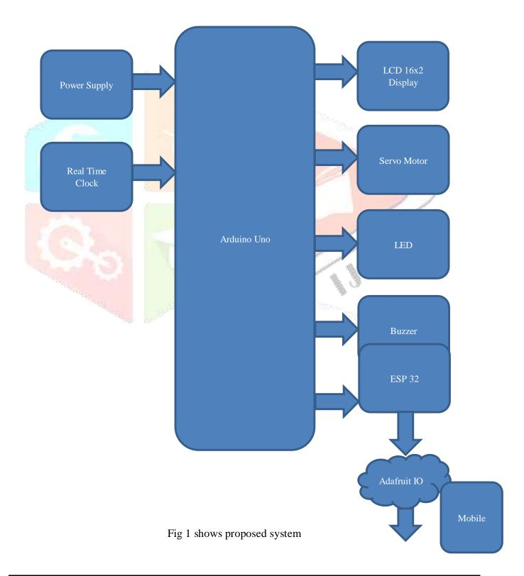
The proposed **IoT-based Smart Medicine Dispenser** consists of interconnected hardware and software components that work together to automate medication dispensing, provide reminders, and enable remote monitoring. The **overall block diagram** is as follows:
