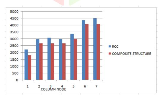
Comparision based on displacement on both structures
