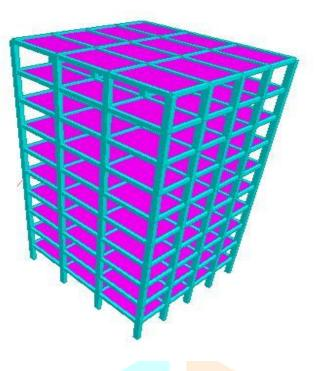
Figure . Rendering view (G+8) RCC building model
