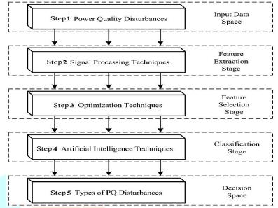
Fig 2: Block diagram of PQ Disturbances Detection and Classification System
