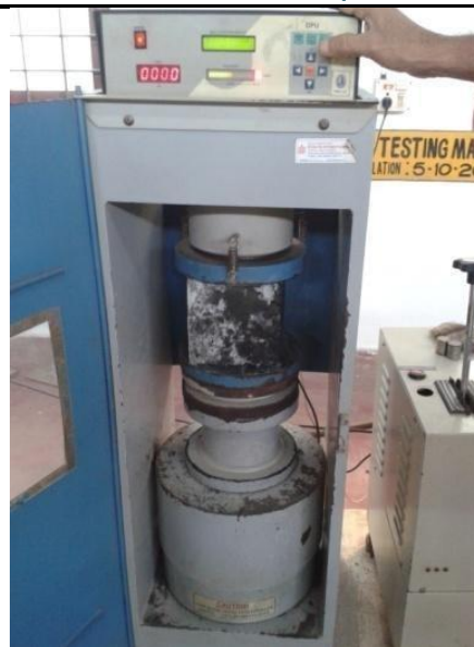
Compressive strength test on cubes
