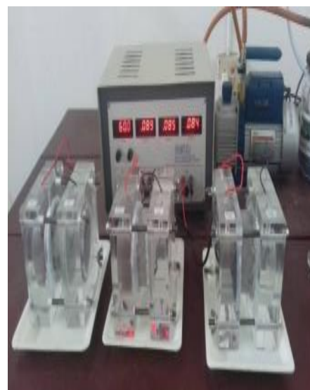
Fig. 3.7 Rapid chloride permeability apparatus
