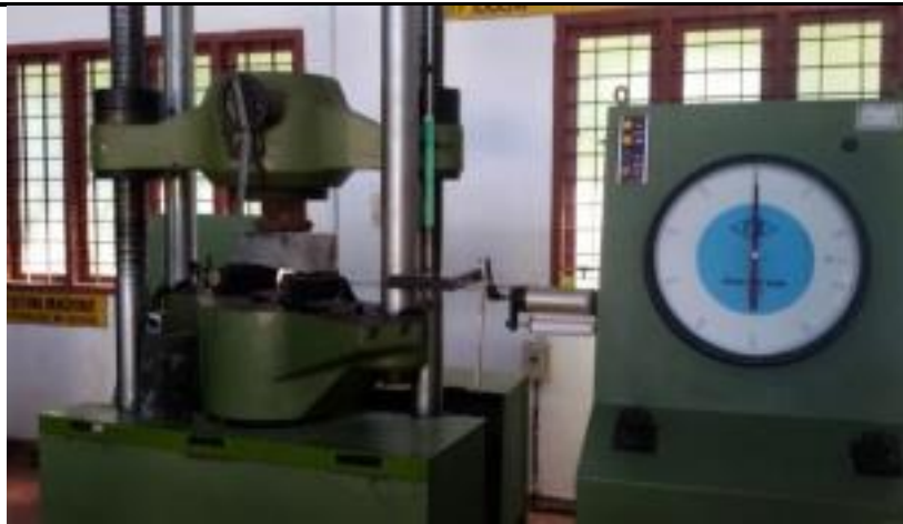
Fig. 3.5 Flexural Strength Test on Concrete Beam
