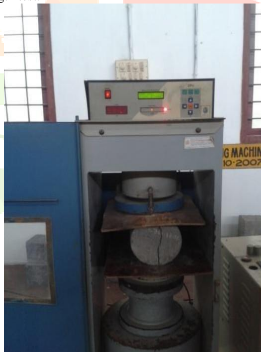
Fig. 3.4 Split Tensile strength test on cylinders
