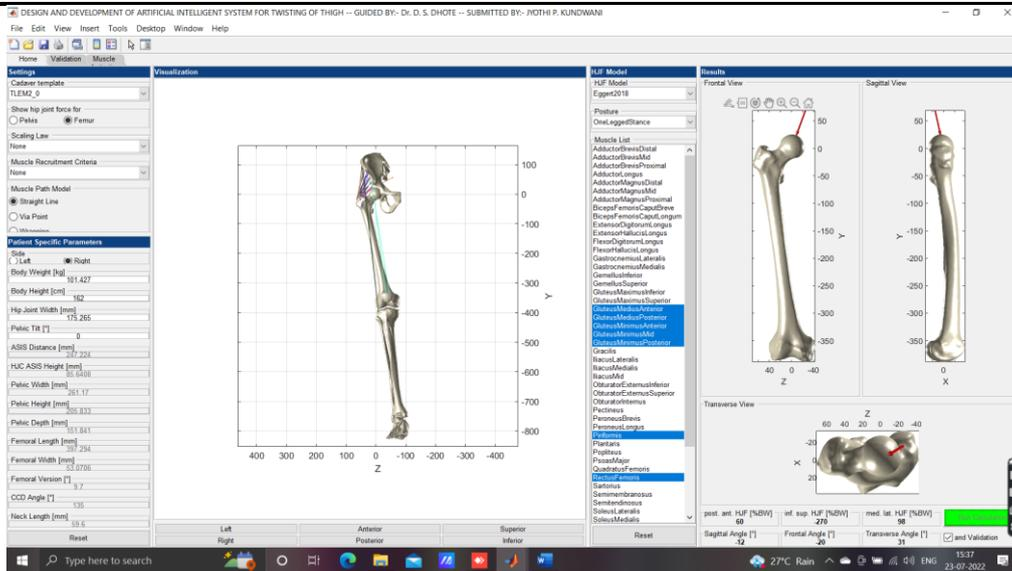
Figure 3:- GUI of hip implant force and muscle selection database
