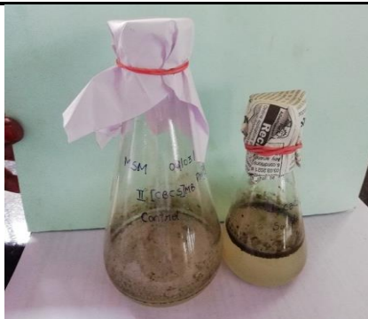
Figure 9: After 28 days, the crude oil biodegradation Saccharomyces cerevisiae
