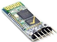
BLUETOOTH MODULE –Bluetooth module is used for wireless communication. This was designed to replace wire cables. This uses serial communication with electronics. This module is usually used to connect small devices. to be operated within 4-6v of power supply. It supports 9600, 19200, 34800, 57600 baud rates. This can be operated in master-slave mode which means it will neither send nor receive external data.
