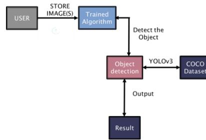
The user data is given as input and it will get processed and segmented by CNN. The objects are detected with help of YOLO and COCO, a bounding box is drawn around the objects along with label to get a labelled output image, while when a video/webcam is user data the system runs/iterates throughout the frames of the video/webcam and again the bounding box along with labels is displayed.
