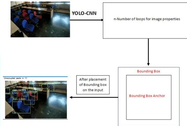
To enter into the system, user needs to pick an image from the device and with the use of OpenCV library read the image and create borders with the help of OpenCV library and also we resize the image to 1080x720 pixels and feed the byte array to CNN algorithm, the CNN then check for the prediction accuracy of greater 0.50(50%). Later YOLO fetches the object name from COCO.names to label the bounding box and display it as output.
