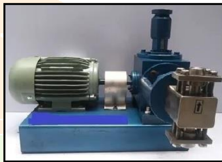
Figure 6.2.4 Feed pump for Decanter Centrifuge
