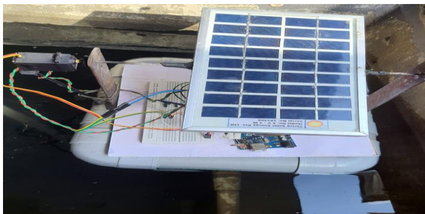
Figure.7 Prototype of floating solar panel with sun position tracker
