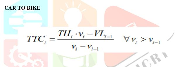
Where, Total Vehicle headway(TH<sub>i</sub>) =1.56, car speed ( $v_i$ )= 36.61 kmph, bike speed( $v_{i-1}$ )=27.63, standard vehicle length of car(VL<sub>i-1</sub>)=3.7m, so as per the formula,
