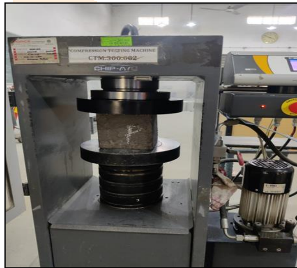
Fig no.2: Shows the testing of Concrete Cubes by CTM
