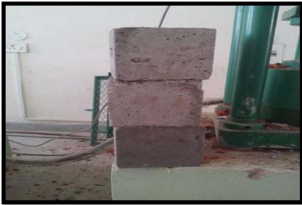
Fig 5.1: Geopolymer concrete cubes ready for testing
