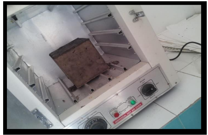
Fig 5.2: Geopolymer concrete cube during heat curing in oven
