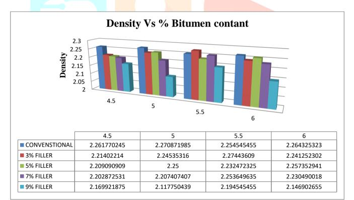
Figure 2 Density Vs % Bitumen contant
