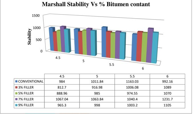
Figure 1 Marshall Stability Vs % Bitumen contant
