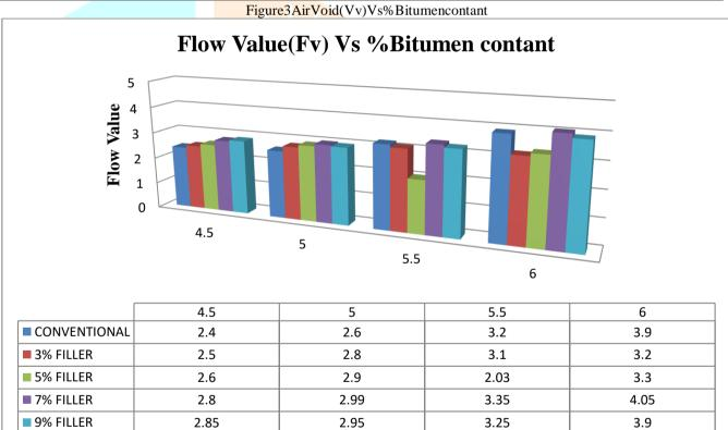
Figure 4 Flow Value(Fv) Vs % Bitumen contant
