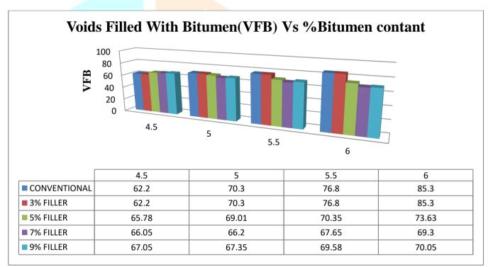
Figure 6 Voids Filled With Bitumen(VFB) Vs %Bitumen contant
