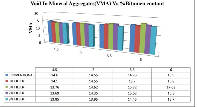
Figure 5 Void In Mineral Aggregates(VMA) Vs % Bitumen contant
