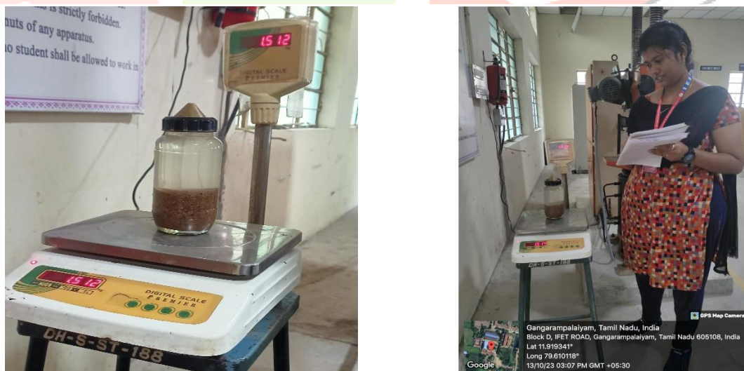
Fig 5.3 SPECIFIC GRAVITY OF FINE AGGREGATE
