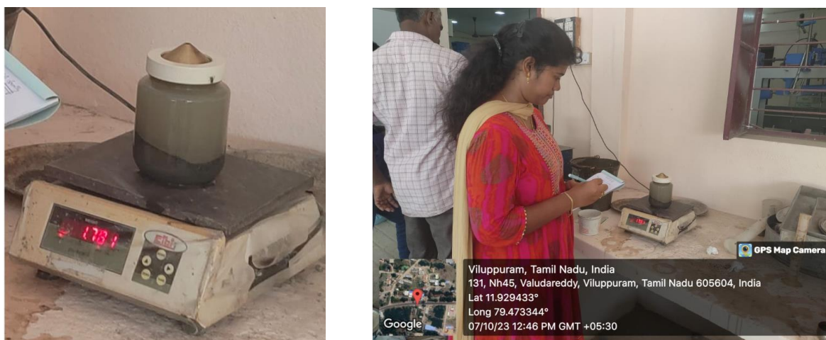
Fig 5.1 SPECIFIC GRAVITY OF CEMENT
