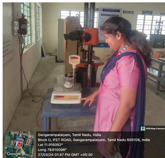
Fig 5.5 SPECIFIC GRAVITY OF PUMICE STONE
