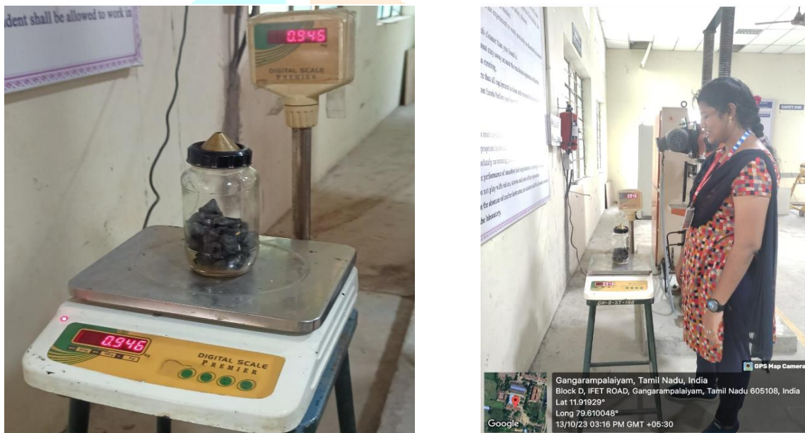
Fig 5.6 SPECIFIC GRAVITY OF COARSE AGGREGATE
