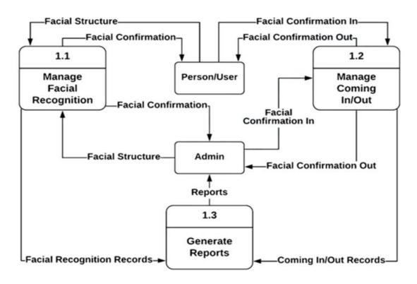
Fig 3.3: Level 1 Diagram
