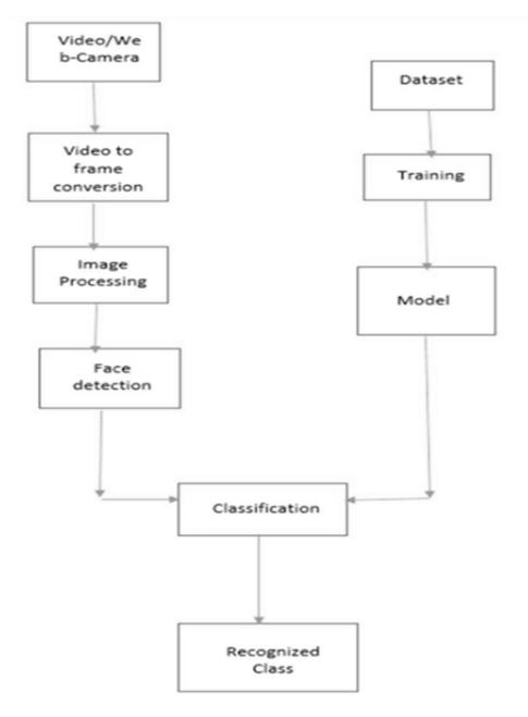
Fig 3.5: Block Diagram
