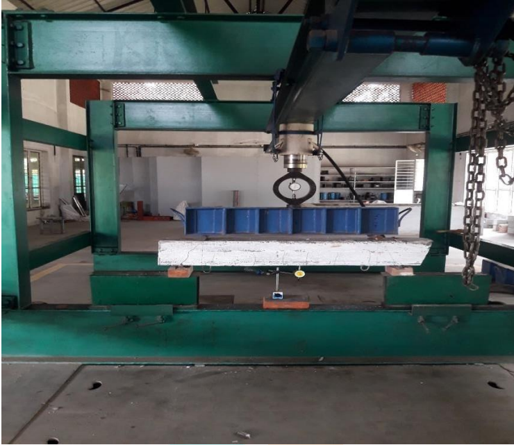
Fig. 5.6 Test Setup for Loading Specimens
