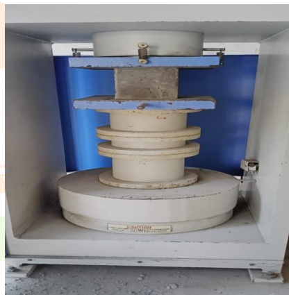
Figure F.7 Compressive Strength Test of SCC Mix with CS AND EFBF
