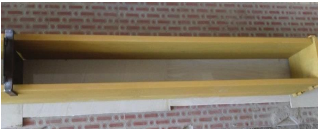
Fig. 5.1 Mould for Beam Specimen
