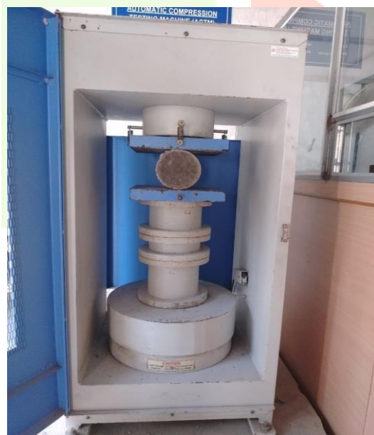
Figure F.6 Split Tensile Strength Testing of SCC 30 Mix with PPF
