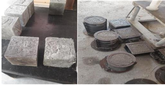
Fig. 5.1 Casting of SCC Specimens
