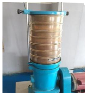
Fig. B. 1 Sieve Analysis
