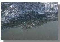
Liquefaction in sand layers, and in sand and silt seams in the clayey soils beneath Anchorage, caused many of the destructive landslides that occurred during the
