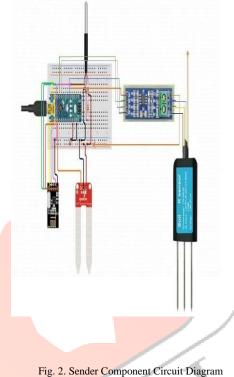
1) Arduino: Arduino is an open-source electronic software. The board has been used for many applications like read inputs activating a motor, turning on an LED and so on. In this case we are using an Arduino nano with an operating voltage of about 5V and recommended input voltage for Vin pin around 7V-12V. It has flash memory of 32Kb and 2kb is used for bootloader.
