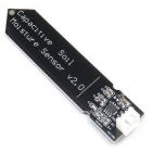
Fig. 4. Capacitive Moisture Sensor
