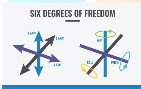
Based on this principle the Gyro sensor also known as angular rate sensor, used to The Gyro scope helps in determining the moment on hand gesture, this sensor is used to measure angular velocity, hence such moments like Roll, Pitch and Yaw. Along with flex sensors are used to detect sign language. The values of Gyro range from  $\pm 125$ ,  $\pm 245$ ,  $\pm 500$ ,  $\pm 1000$ ,  $\pm 2000$  degree per second (DPS).
