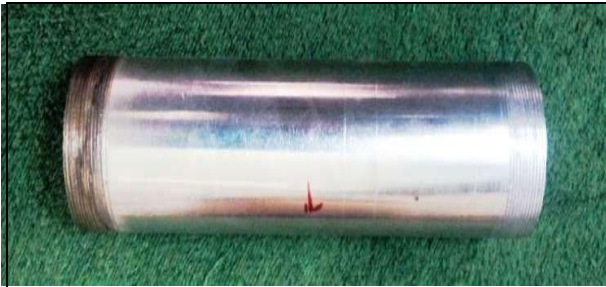
Figure 5: Damper Cylinder (Housing or Shock Tube)
