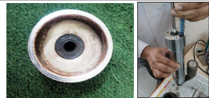
Figure 8: Upper end cap with seal and filling of damper
