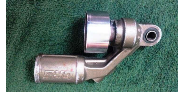
Figure 7: Accumulator with lower end cap
