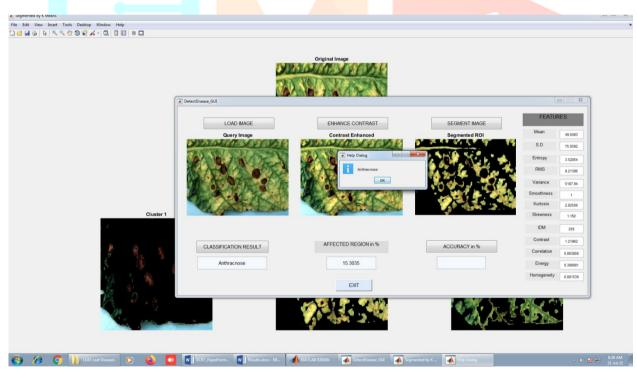
Further this binary image is given to neural network for classification, it is inferred that the leaves which are affected by diseases shows significant differences in their neural output when compared to the normal leaf. Furthermore, the disease categories can also be easily categorized. Hence we have successfully classified the disease
