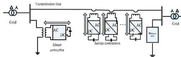
The central control unit generates reference signals for the shunt and series converters of the DPFC to regulate the bus voltage and to control power flow in transmission line. All the reference signals generated by the central control unit are corresponded to the fundamental frequency components.
