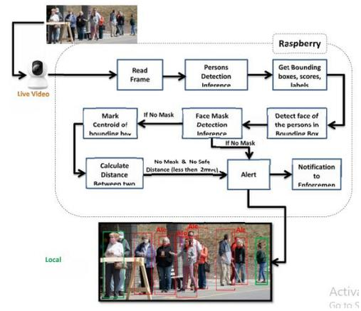
The proposed system uses a transfer learning method using an in-depth learning algorithm with a computer the idea of automatically monitoring people in public places with a camera and finding people with a mask or no mask. We also make good order, which is another way to learn to transfer, much more powerful than feature removal.
