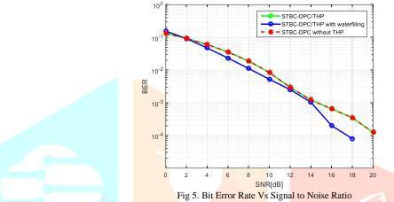
This simulation result evaluate the BER performance for the STBC-DPC systems. Figure 4. shows the output BER curves. It is observed that the STBC-DPC/THP with water filling Algorithm can provide better performance than the STBC-DPC/THP and STBC-DPC systems at SNR>24 dB.
