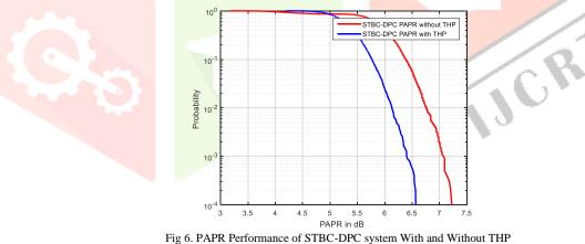
Figure 5 shows the PAPR of STBC-DPC system with THP is demonstrated. It shows that the STBC-DPC with THP system
