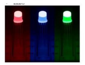
LED is an active electronic device, comparable to a general purpose diode except for its ability to emit light with different wavelengths. When a suitable potential difference is applied across its terminals, electrons recombine with the holes within the device thereby releasing the energy in the form of photons. This phenomenon is known as electroluminescence.
