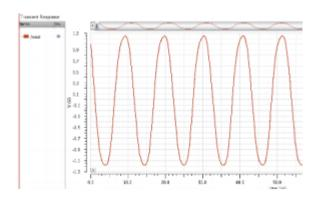
Fig 6 resultant wave form of the ring oscillator
