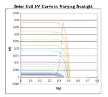
Photovoltaic solar cell I-V curves where a line intersects the knee of the curves where the maximum power transfer point is located.
