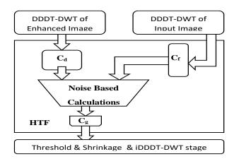
Fig 1. Block diagram of Noise based Hybrid Threshold factor Calculation
