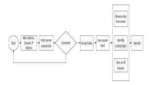
Arduino Microcontroller is Connected to Wi-Fi module and Relay Module. Relay Module are going to be further connected to devices and appliances. Home Devices are controlled through mobile using application. Application will take the dynamic IP address, accept data, user provide the input through on/Off button, through which the sensor will identify the device to regulate and execute.
