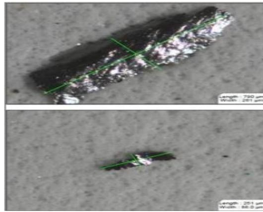
The microscope system can divide particles into reflective particles and non-reflective particles to indicate the ratio of metallic particles to non-metallic particles. In order to analyze contaminants in depth, the particles can be analyzed using the XRF microscopy – which can accurately identify the particle type and its correlation with the possible source (1).
