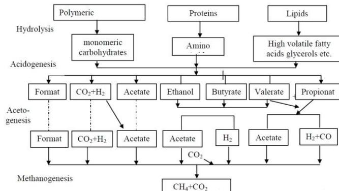
**4. Methanogenesis:** In this final step methane is formed by methanogenic bacteria metabolize acid, alcohols, carbon monoxide, carbon dioxide and hydrogen into Methane. The methanogenic bacteria are sensitive to the environment as they only work in a strict anaerobic condition.
