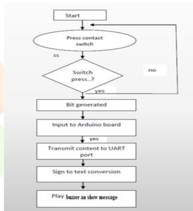
Fig.1: Working flow chart of the smart gloves
