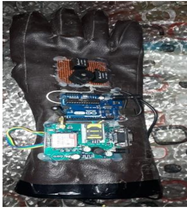
Fig.3: Final product showing all the associated electronics of the smart glove
