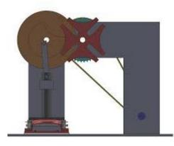
4) **Punching ram**: Punching is performed by moving the sheet metal between the top and bottom tools of a punch. The top tool (punch) mates with the bottom tool(die), cutting a simple shape (e.g. a square, circle, or hexagon) from the sheet by using punching ram and die. IJCR
