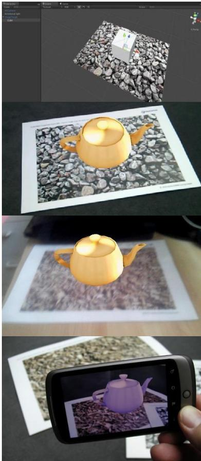
This image represents the initial marker tracking of object over the image target item. Here, we are initializing the position on the target image for the virtual object to be overlaid.
