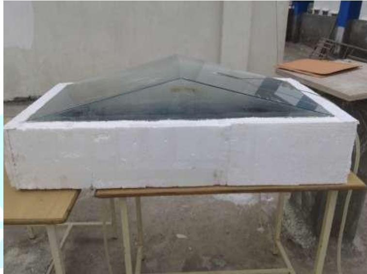
Figure 3: Experimental setup of non-conventional double slope solar still
