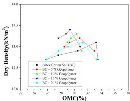
**Compaction characteristics of various percentages of geopolymer treated with expansive soil**
