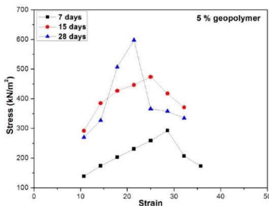
**Unconfined compressive strength of expansive soil in the curing period of 7,15&28 days treated with fly ash based geopolymer**
