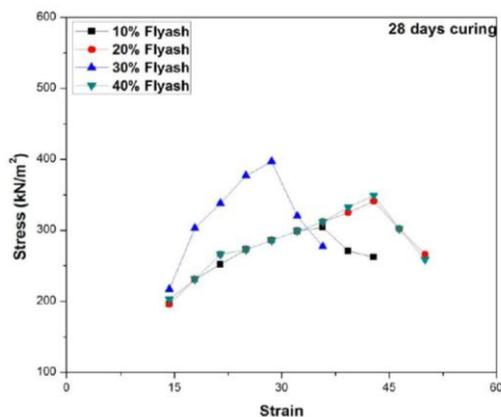
**Unconfined compressive strength of expansive soil treated with various percentage of fly ash in 28 days curing period**
