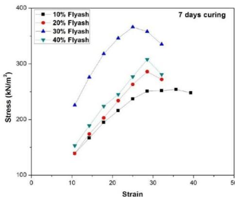
**Unconfined compressive strength of expansive soil treated with various percentage of fly ash in 7 days curing period**
