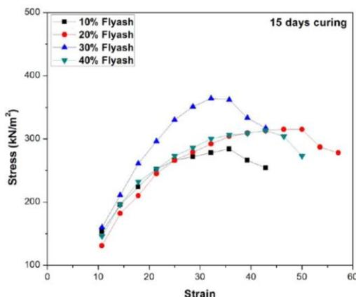
**Unconfined compressive strength of expansive soil treated with various percentage of fly ash in 15 days curing**
