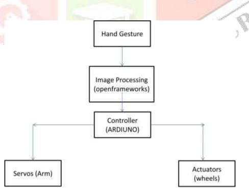
The overall block diagram of the setup is given in the Fig. The hand gestures are read as images through the camera attached to the wheelchair. Then, they are processed by the algorithm and then a control character is sent to Arduino by serial communication. The Arduino controls both the arm and the wheelchair based on its reception of the control character.
