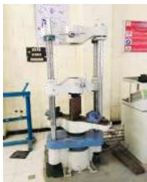
Fig 4. compressive strength perpendicular to surface in UTM
