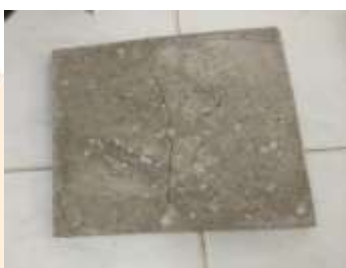
Fig 9. Shows the failure state of the specimen when subject to flexural
