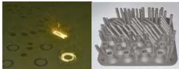
Fig. 16. SLM-exposure of the specimens (left) and generated specimens on the substrate plate (right).
