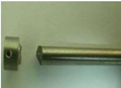
Fig.21 Fracture portion of the bolt
