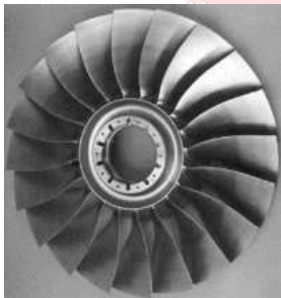
Fig. 8. Titanium blisks for compressor applications (MTU Aero Engines, Munich, Germany).
