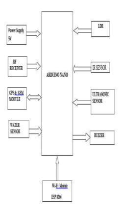
We planned a system which consists of a microcontroller, LDR sensor, IR sensor, ultrasonic sensor, water sensor, GPS and GSM module, RF transmitter and receiver, Wi-Fi module and a buzzer. Software part of our planned system are coded in
